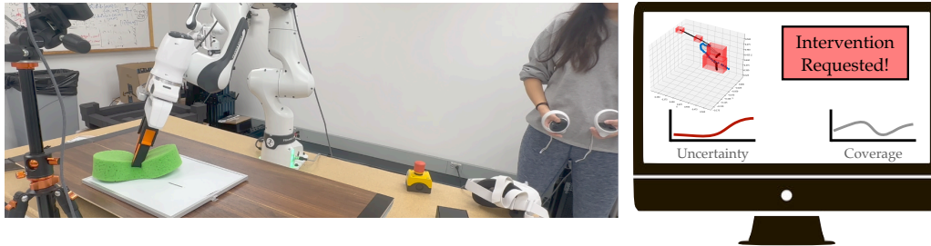
Figure 12: When the robot needs help, the robot pauses its execution and presents an alert notification on the screen.
